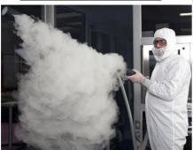
the Clean room environment. The <u>high density fog increases the duration</u> <u>and travel distance</u> of the fog. Enclosure is a high impact, white powder coat
