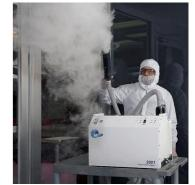
It is used to visually track air flow direction and velocity, to insure an even flow split from the clean room bays into the adjacent equipment chase and to detect unwanted air infiltration into a clean room. UltraPure Foggers are used in Pharmaceutical Processes to prove process environments are operating properly, as
