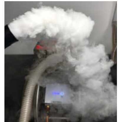
Dense Fog To Visualize Airflow
